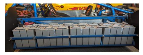
The EVSR Power System is a "Floating" System which means the High Voltage (HV) circuit grounds are separate from the Low Voltage (LV) circuit grounds. The Computerized Controller System (CCS) measures the HV system's "Isolation" from HV Circuits to Chassis Ground. Faults will be displayed in the Driver Instrument System (DIS) / Cluster. An electric shock may occur if the HV circuit ground is shared with the LV circuit ground.
