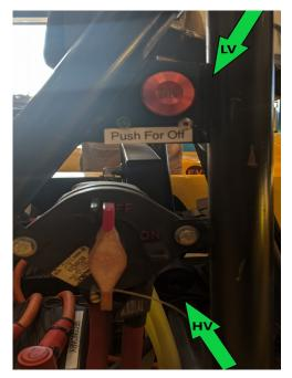
This switch may also be turned off by pulling the loop or T handle to Drivers Right of the instrument panel.
